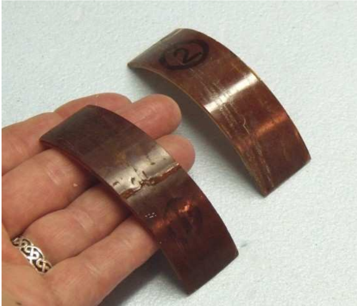
Figure 3. An image of the tested Ameron tube specimen after buckling under the force during heating [left] compared to an untreated sample [right].
