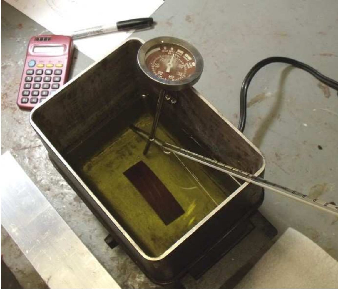
Figure 1: Experimental setup with the sample immersed in the oil. Top view.
