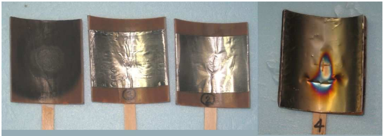
Figure 4 – Condition of specimens after exposure to flame (#1-4, left to right)
