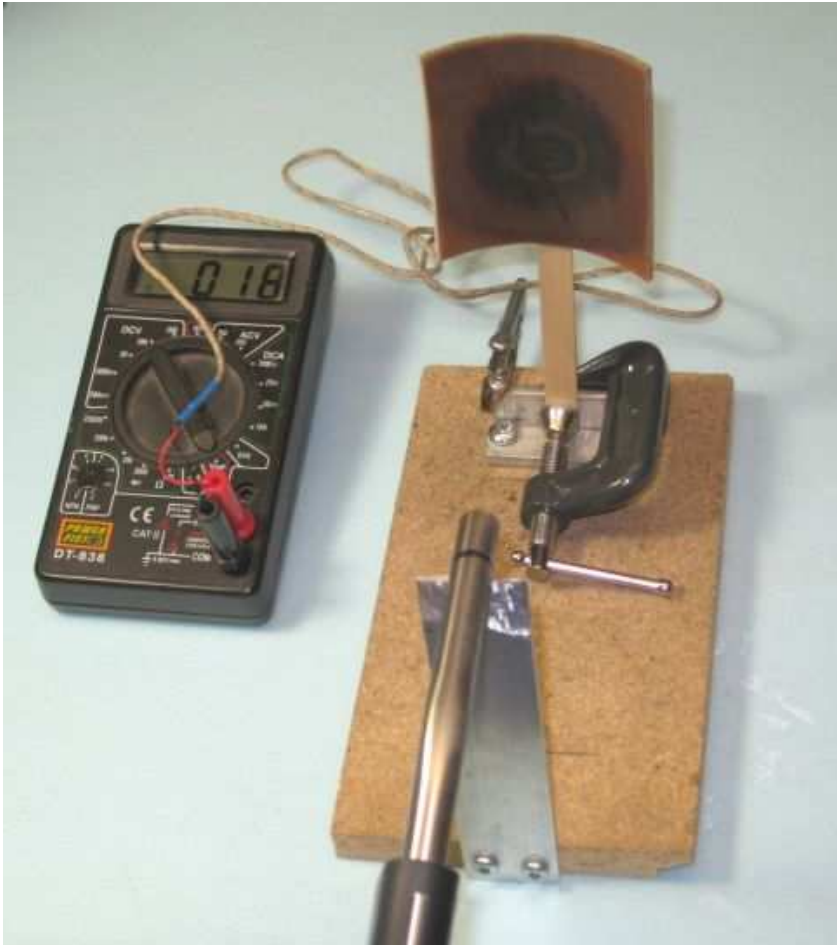
Figure 2 – Setup for application of flame heating to specimens
