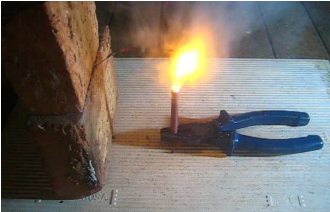
Fig. 9 Successful strand burn rate test
