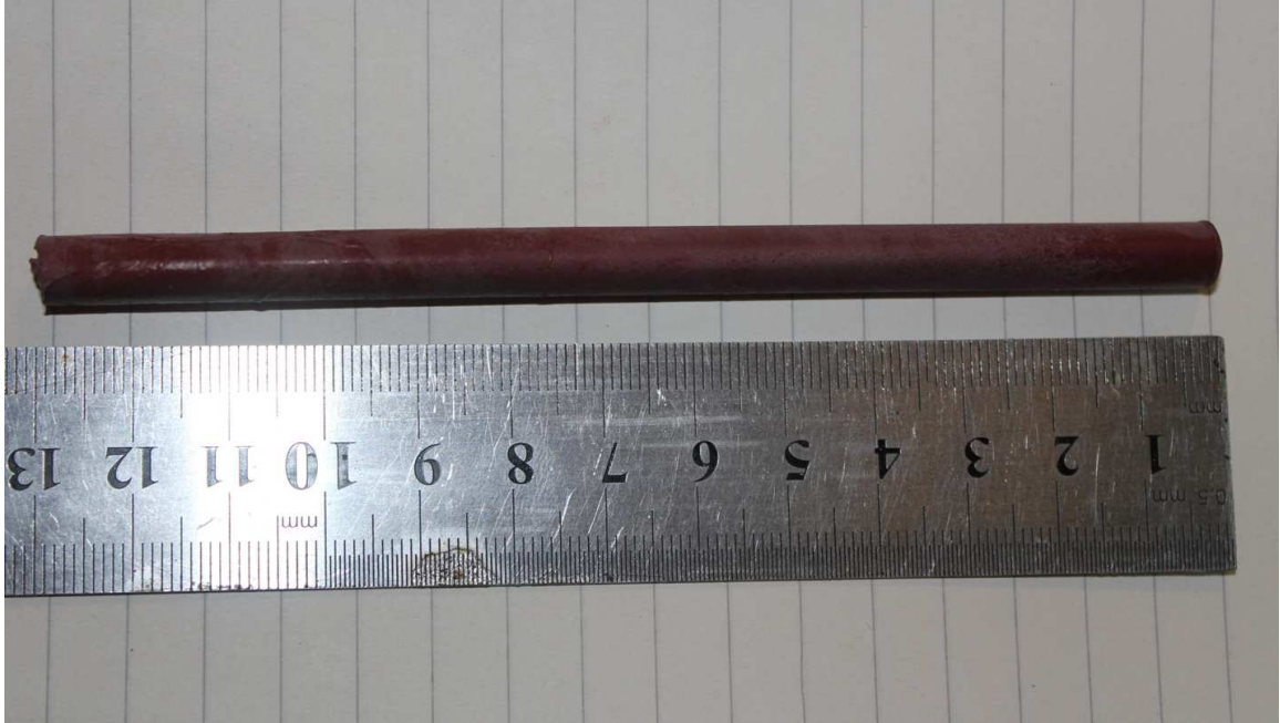
Fig. 8 Cast KNO_3 - NaNO_3 -Mannitol strand with red iron oxide additive
