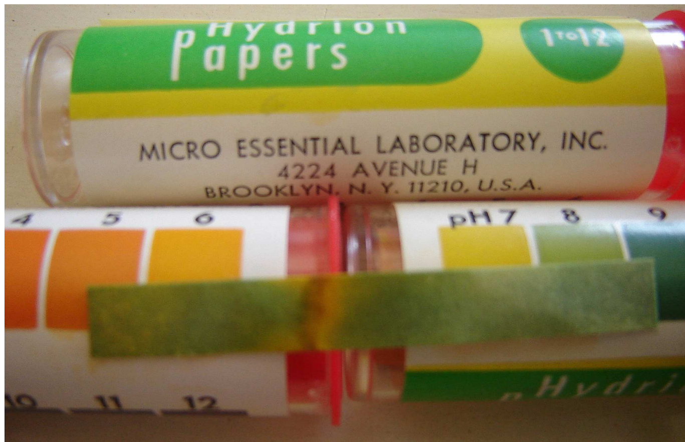
Figure 1 pHydrion pH strip test of “Shanxi Wencheng Chemicals Company” \text{KNO}_3
