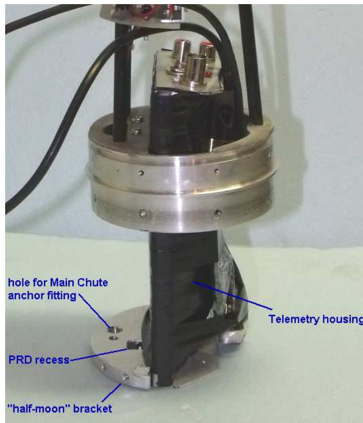
Figure 3 – Bracket for attaching main chute anchor and PRD
