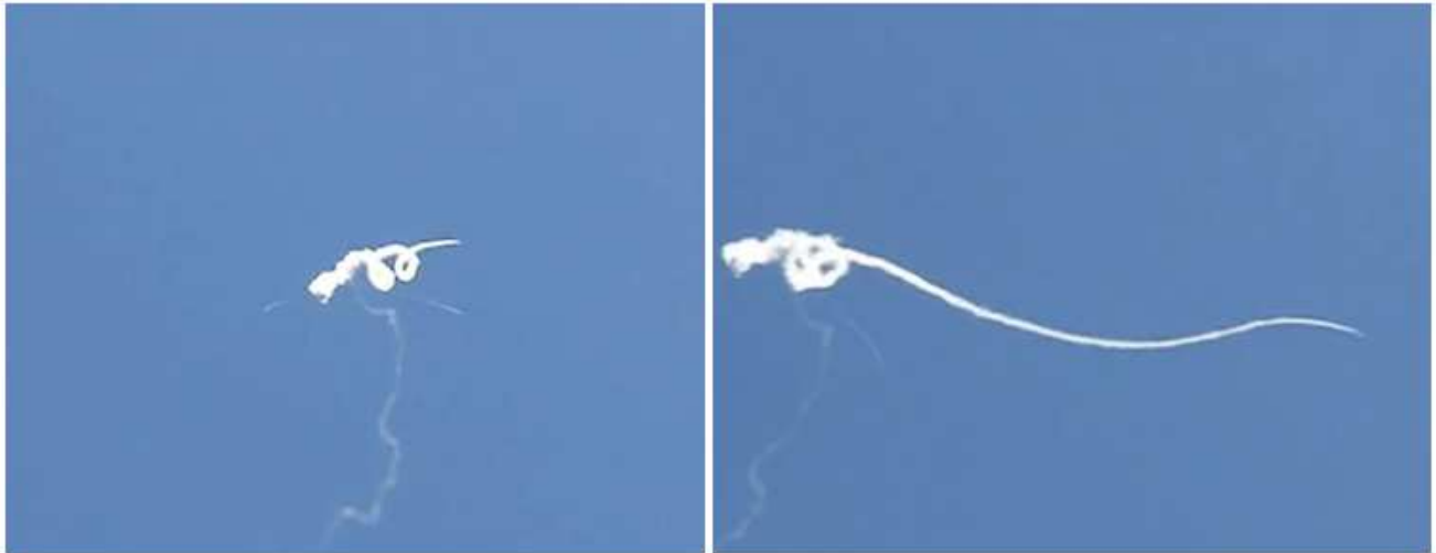
Photo 13 – Shortly after anomaly, vehicle loops twice, then trajectory straightens out
