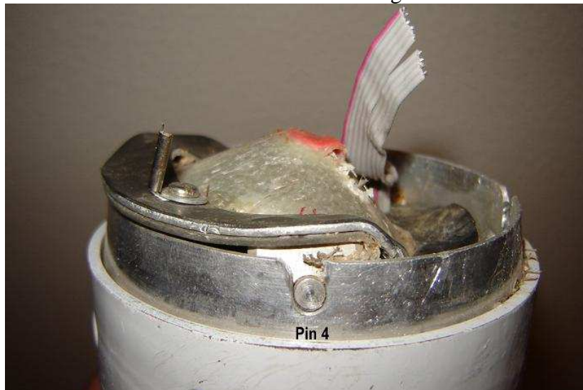
Photo 26 – Coupler shear tear-out damage at PSD retention pins
