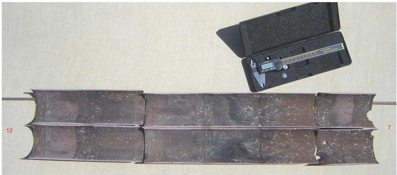
Photo 23 – Forward casting tubes after cleaning and splitting open for examination
