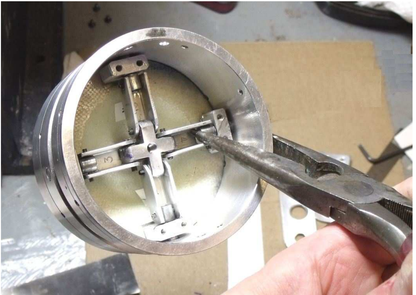
Figure 2 - Using pliers to extend pins fully outward
