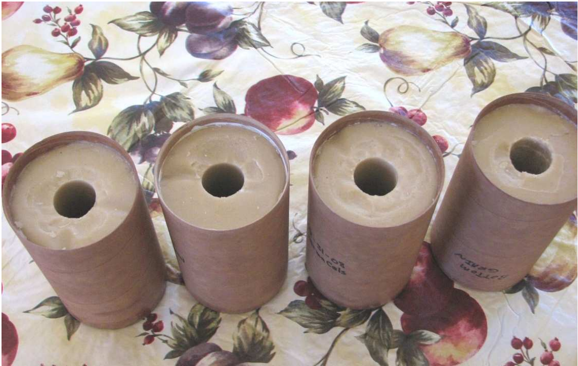
Figure 3 – Bottom surfaces were chipped during coring rod removal.
