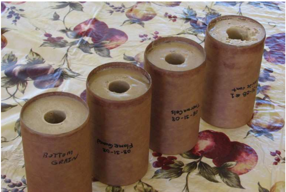
Figure 4 – Irregular propellant top surfaces.
