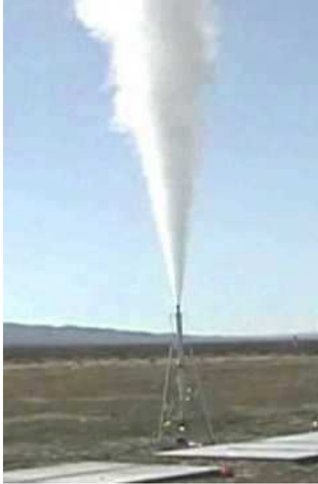
Photo 4 – 1 st phase motor undergoing full thrust
