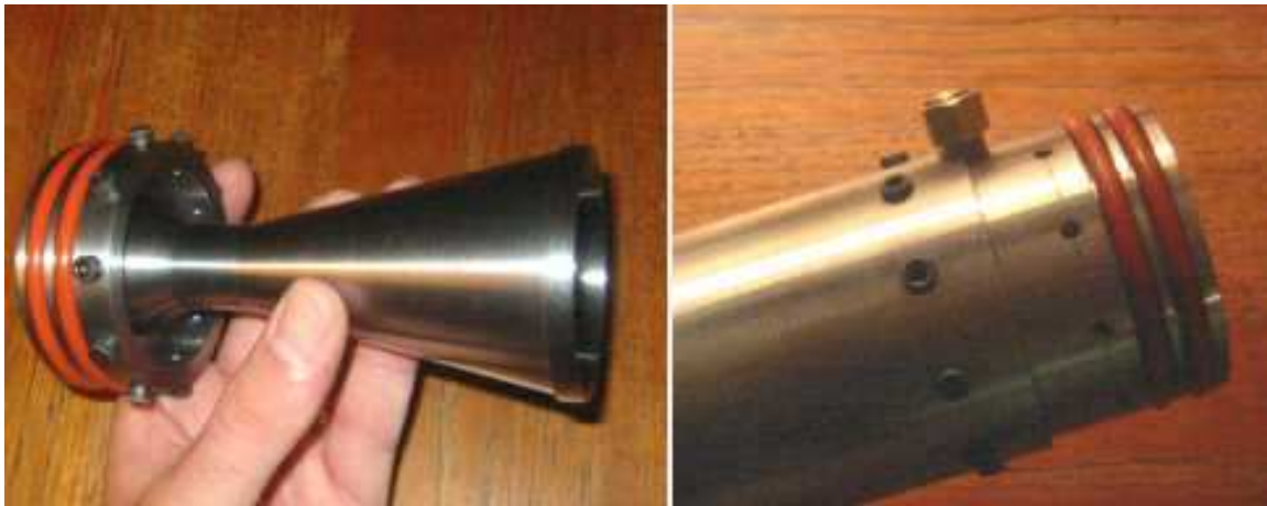
Photo 2 – Nozzle (left) and installed mid-bulkhead (right)
