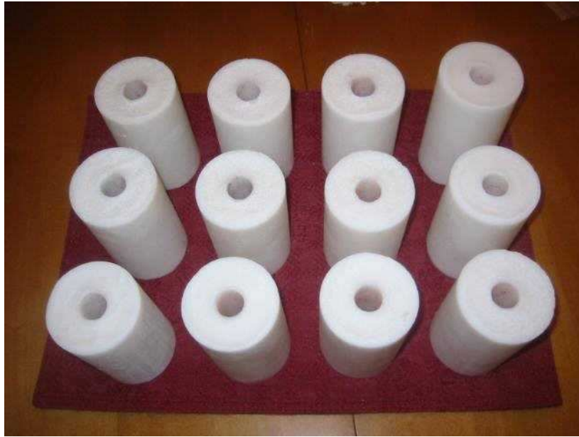
Photo 1 – Propellant grain segments prior to inhibiting
