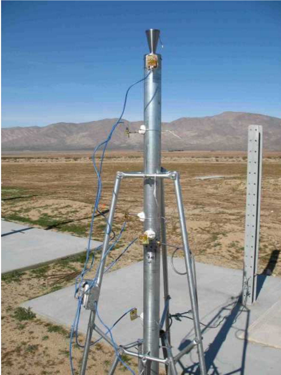
Photo 3 – Instrumented \frac{1}{4} Scale BEM in static test stand
