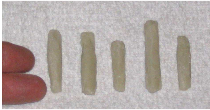
Fig. 7 - Propellant strands for burn rate measurements, prior to painting.
