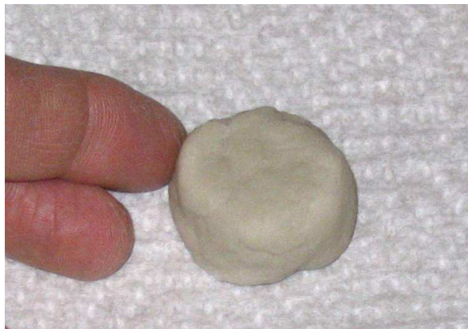
Fig. 8 – A small sample of the KNSB propellant produced by vacuum-evaporation method.
