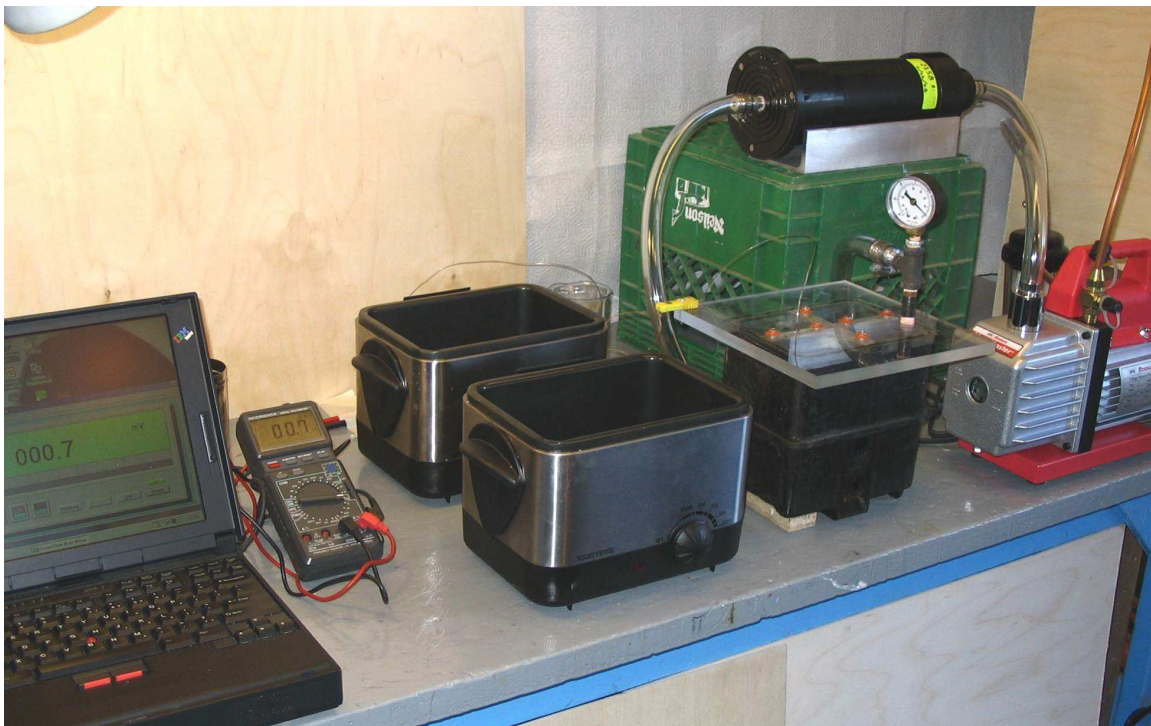
Fig. 2 - Apparatus used in experiment. Left to right: laptop, DVM, Heating unit #1, unit #2, unit #3, vacuum pump. Dessicator is on top of green box.
